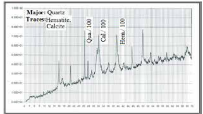
Figure 16: X-ray diffraction pattern of a sample (iron bars of the seaside window) demonstrating quartz, hematite, and calcite.
